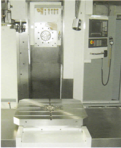
6. 800MM X 700MM BUILT-IN INDEXING TABLE FOR EBM-1000.
